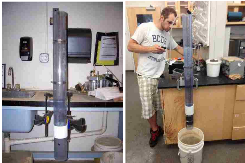
Figure 2.1 Falling head permeameter used for the permeability testing
