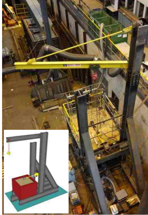
Figure 4.2 Laboratory Soil-Structure Interaction (SSI) testing facility with lateral loading set up and a 3D system sketch (bottom left).
