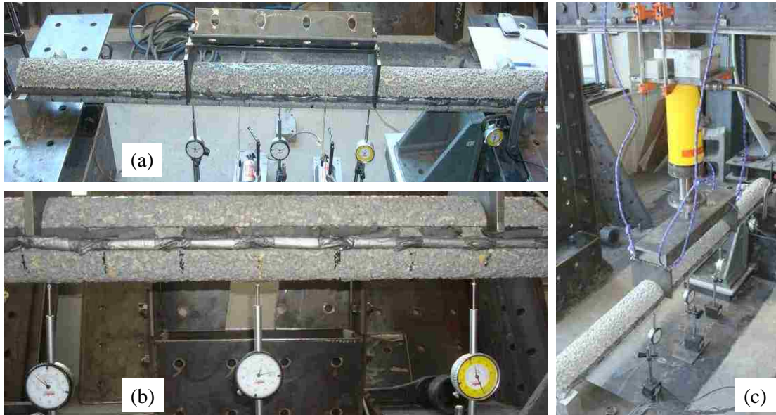
Figure 2.11 Beam test setting up of pervious concrete pile: (a) pervious concrete pile setting up; (b) SAA and dial gauge setting up; (c) hydraulic load on beam
